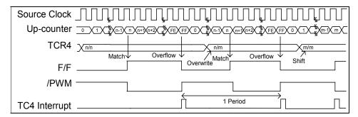
Fig. 5-26 Timing Chart for PWM Mode
